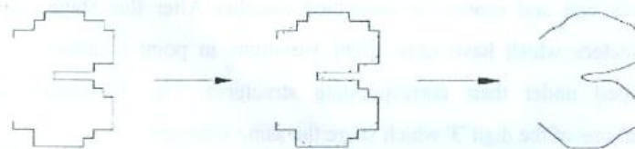
Fig. 11. Eliminating zig-zag line segments during structure extraction.
