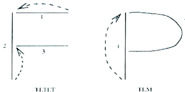
Fig. 4. Examples of some characters encoded using Berthod and Maroy's scheme.
